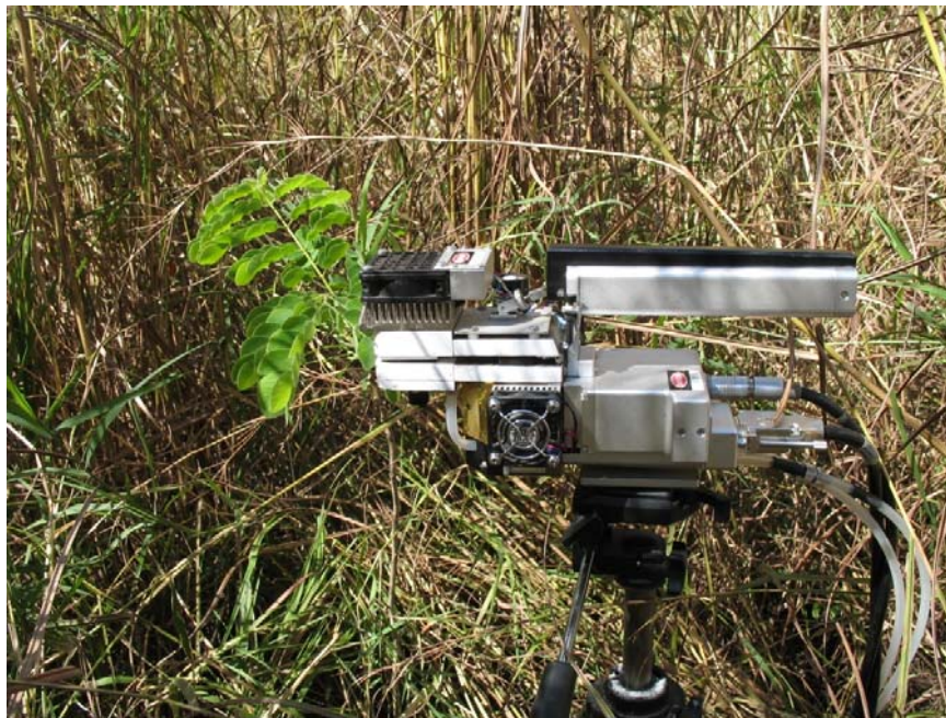
Photosynthesis measurements with LICOR LI-6400.
